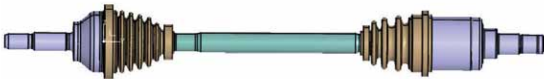
Gelenkwelle links - Vollwelle Ø 21,5 mm
